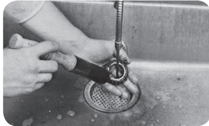
Rinse bearing in clean solvent (fig. 5).
