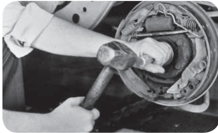
Tap new bearing into shaft cavity (fig. 20).
