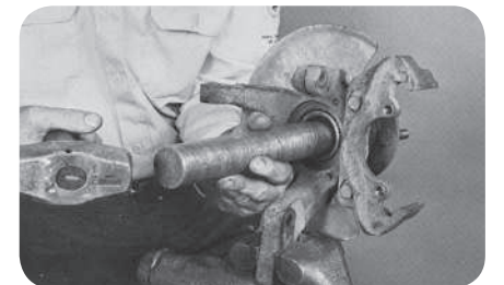
Chrysler – Remove hub from knuckle (fig. 29).
