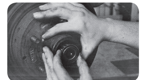
Install outer bearing (fig. 12).
