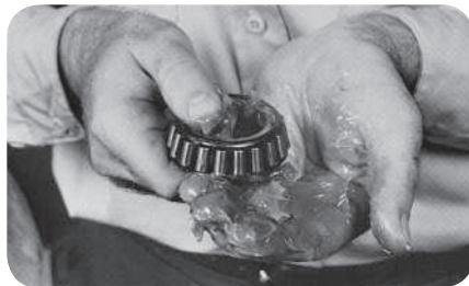
Grease bearing (fig. 7).
