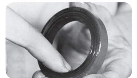
Apply lube to seal lips (fig. 43).
