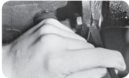
Mark the driveshaft and pinion flange (fig. 39).
