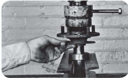
Use arbor press to install bearing (fig. 22).
