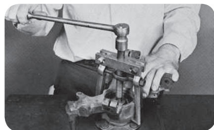
Ford – Grip and remove knuckle from hub (fig. 32).
