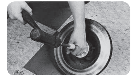
Tap tool until seal is seated in hub (fig. 10).
