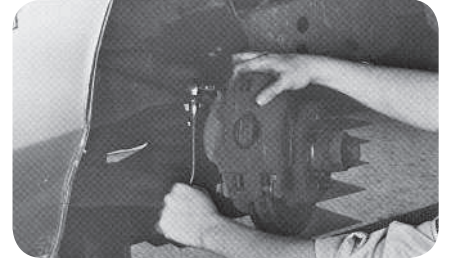
Loosen brake caliper mounting bolts (fig. 1).
