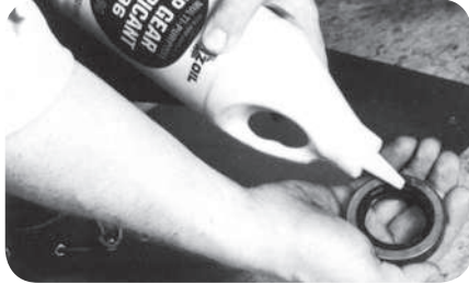
Pre-lube seal with differential lubricant (fig. 19).
