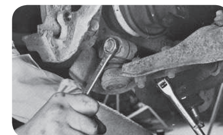
Chrysler – Tighten lower control arm attaching bolt (fig. 36).
