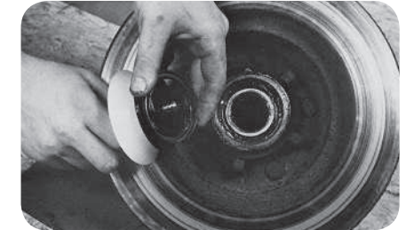
Slide SKF seal onto installation tool (fig. 9).
