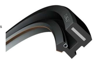
The TR/7/M/PTV differs from TR/7 by the presence of a flexible metal rather than a textile back. The use of a retainer plate as advisable due to the potential pressure in the system.
