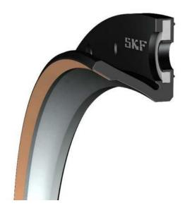
The TFW/PTV seal is characterized by an exclusive PTFE antifriction band vulcanized on the sealing lip – patented with number PCT/EP2006/004962. The PTFE grade is filled according to surface conditions and roughness related to the application. This PTFE band is an integral part of the seal body.
