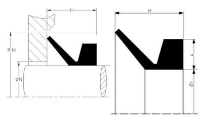
speed exceeding 6-8 m/s requires an axial support, whilst over 10-12 m/s a radial retention is necessary.
