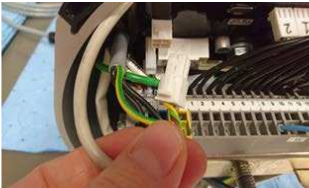
In IF-130 models disconnect the IF-103 wire from the circuit board.
