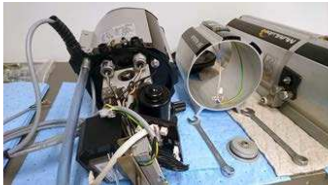
Remove the lower shell with IF-103 user interface.
