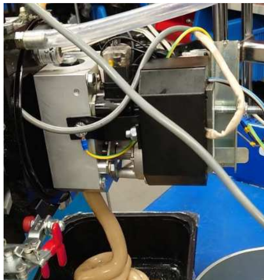
Set the pressurisation time (P) to 999 seconds and start pumping (press SET ).
