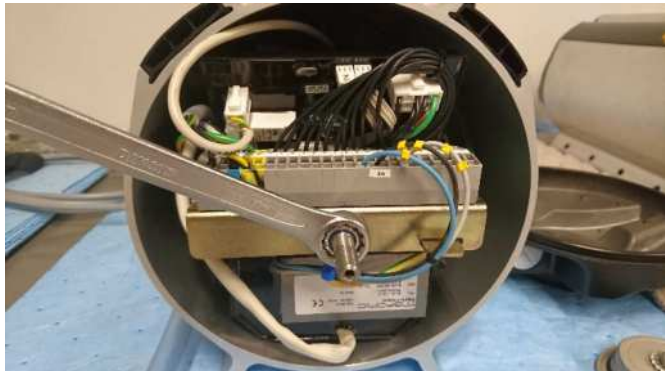
In AC models disconnect the ground wire (17 mm wrench).
