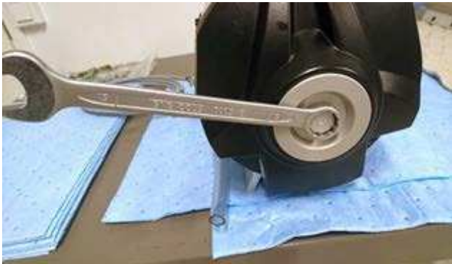
Remove flange nut from bottom (19 mm wrench).
