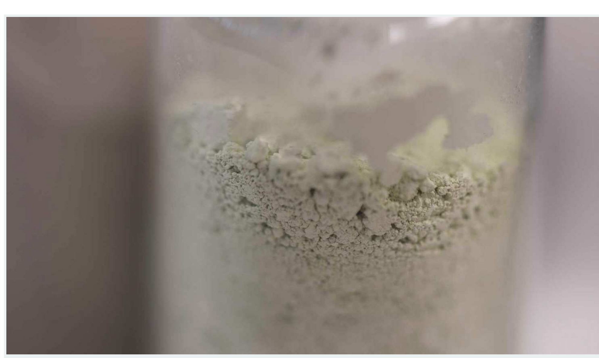
Ceramic components are made by a sintering process where a fine powder of silicon nitride and other additives is milled together and compacted into a shape.
