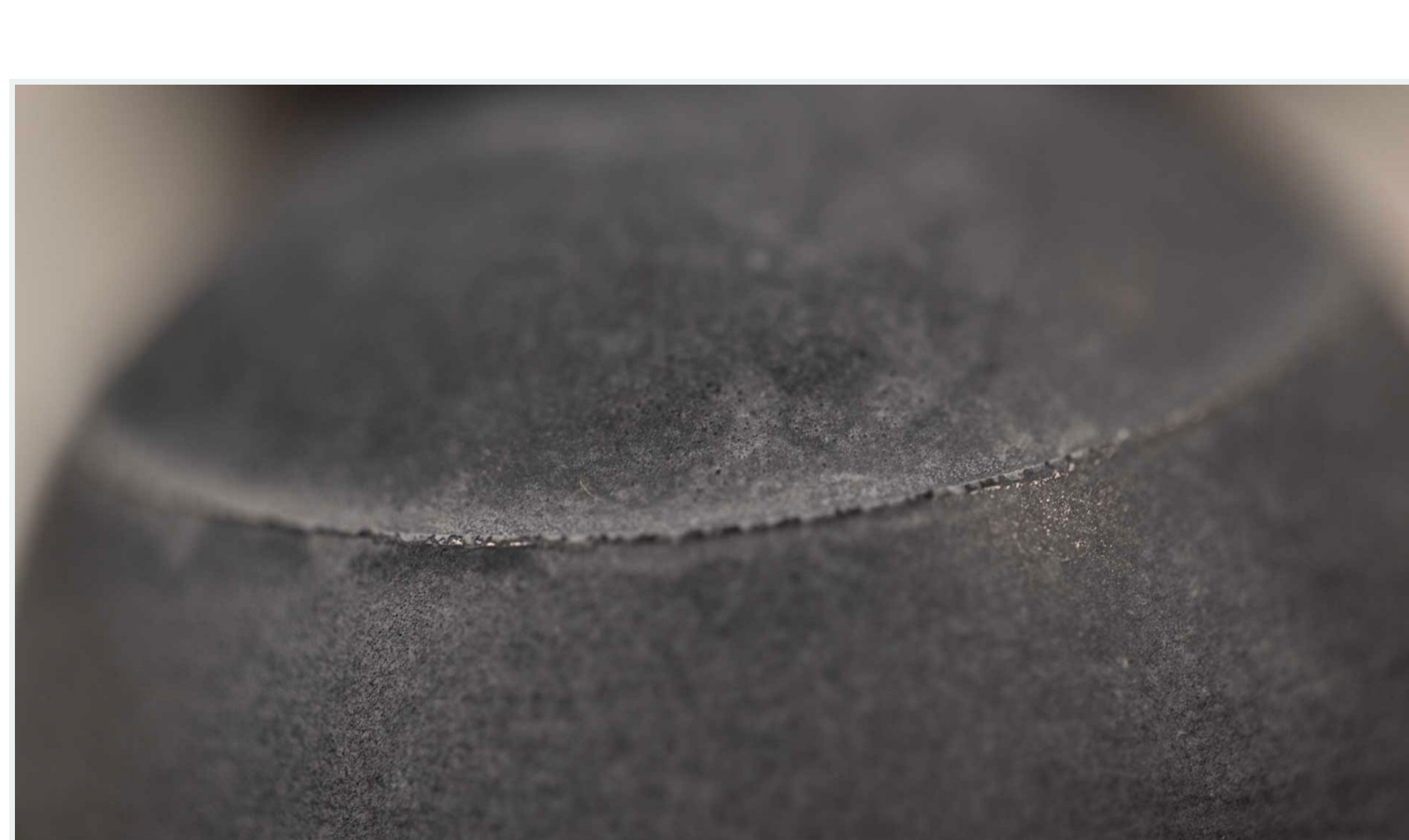
The material is then heated under high pressure until it "fuses" or sinters into a solid, dense "blank".
