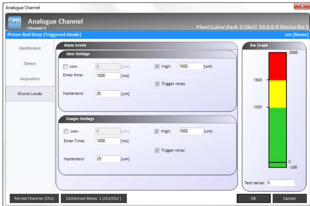
Figure 2 - 135. Configuring Active Alarms and Alarm Parameters for Channel 2.
