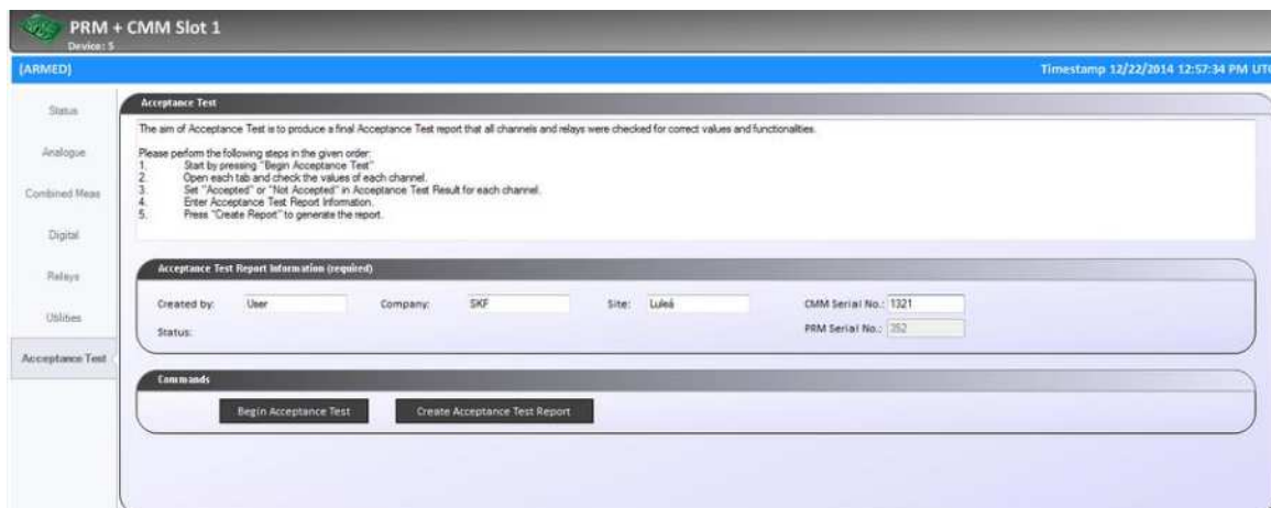
Figure 2 - 66. Maintenance View - Acceptance Test.
