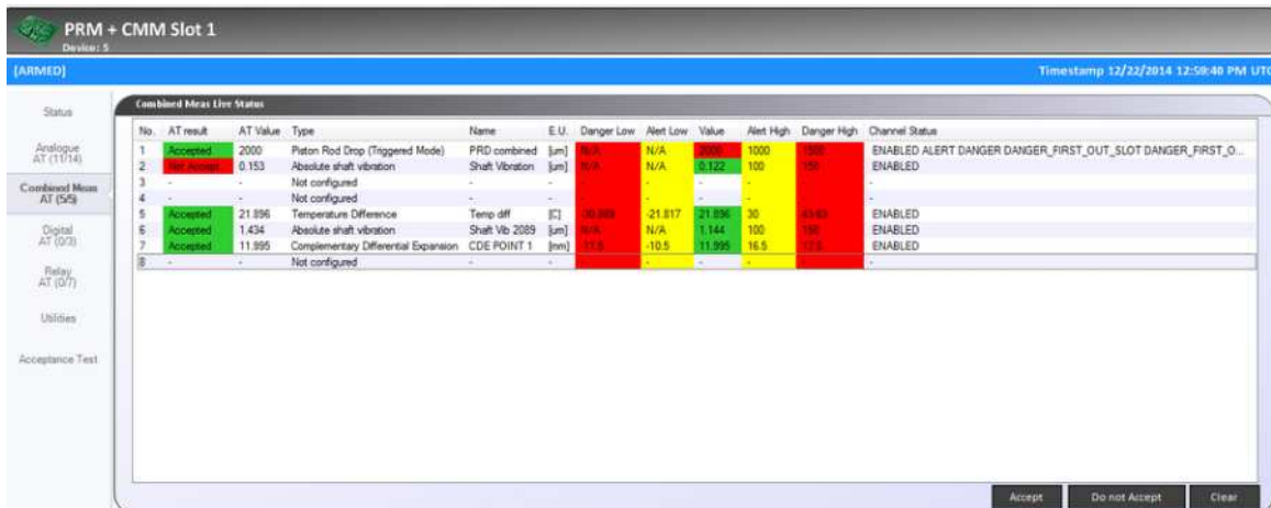
Figure 2 - 68. Maintenance View - Acceptance Test for Combined Measurements.
