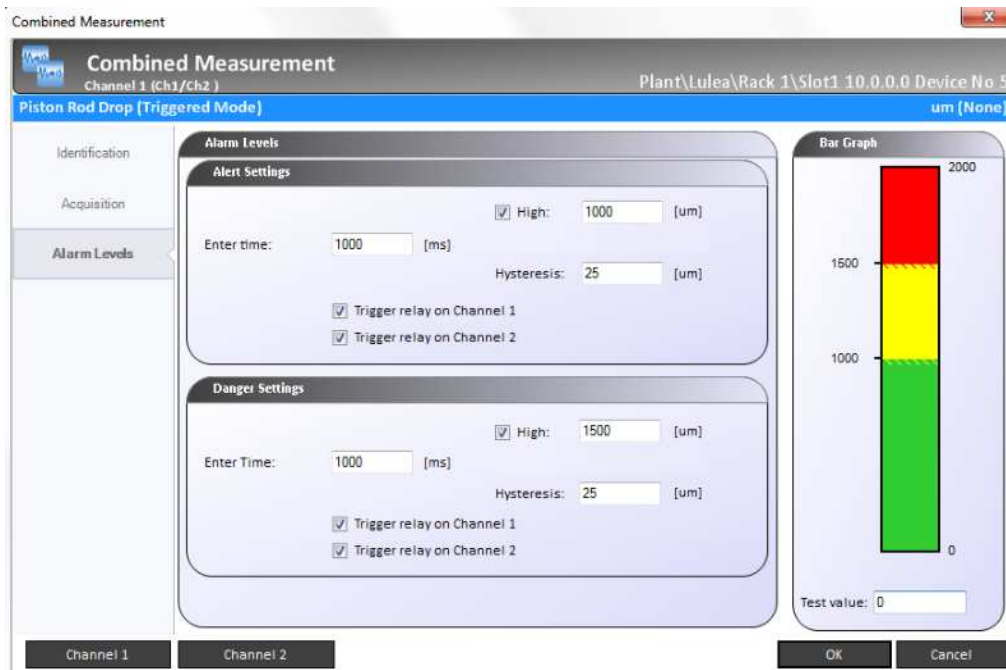
Figure 2 - 138. Alarm Parameters for the Combined Measurement.
