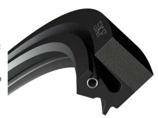
The TR/3/P solid back and lip area provide a good flexibility, to compensate shaft misalignment and a maximum pressure of 0,5 bar. Furthermore, the spring embedding has been carefully studied to prevent its tilting during mounting.
