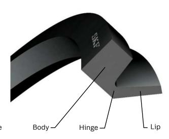
Due to the shape of the sealing lip and the resilience of the polymer used, the TR/VA seal compensates both for angular deviations as well as axial displacement between the shaft and the sealing surface.
