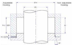
con be restored by adjusting the gland. For a correct housing height, it is recommended to increase H by 2,5 % and use gland shims for a total H of 7,5 %.
