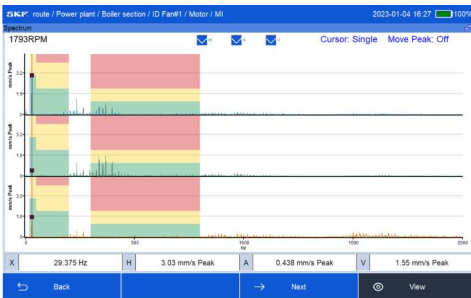
Figure 65 Show / Hide alarm curves
