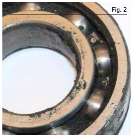
Grease can carbonize and block the bearing at high operating temperatures
