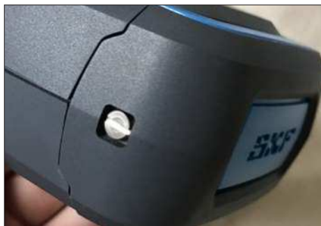
Fig.2 – Compartiment des piles
