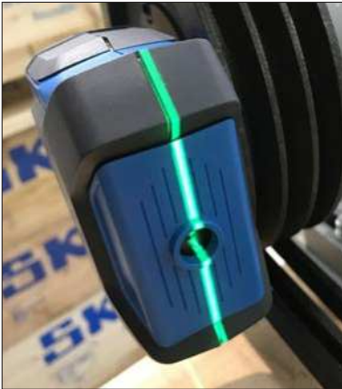
Fig.6 – Display of horizontal angle misalignment
