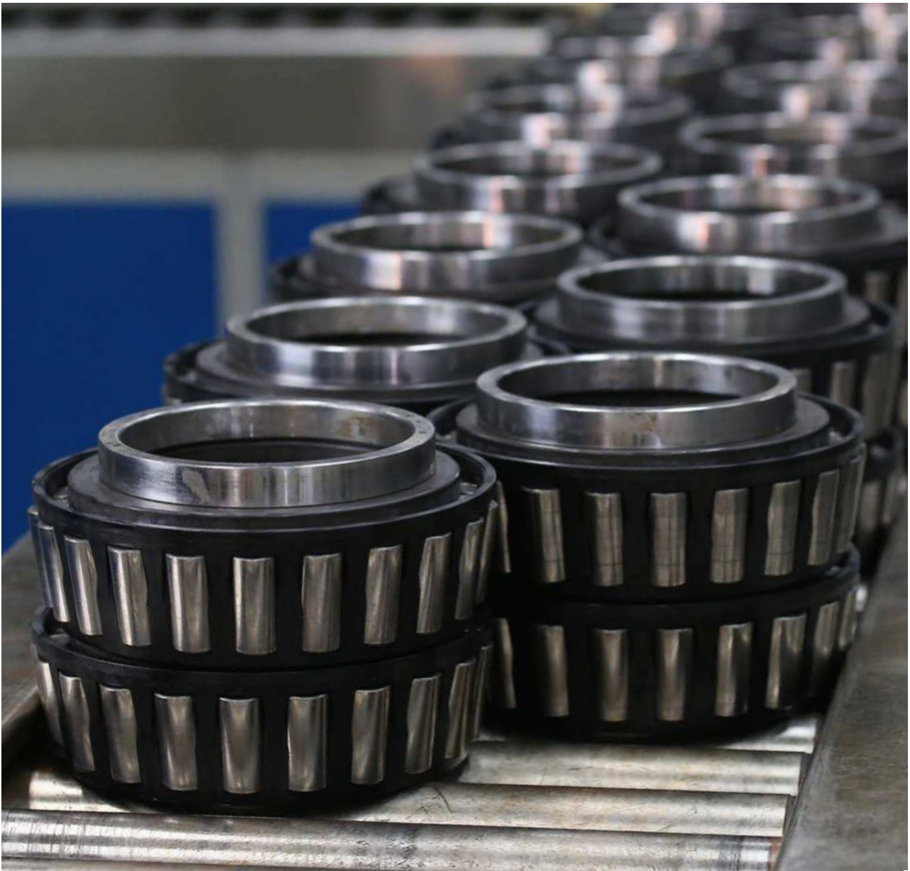
Reuse: Used railway wheelset bearings in the process of refurbishment for extended life at one of SKF Remanufacturing Service Centres
