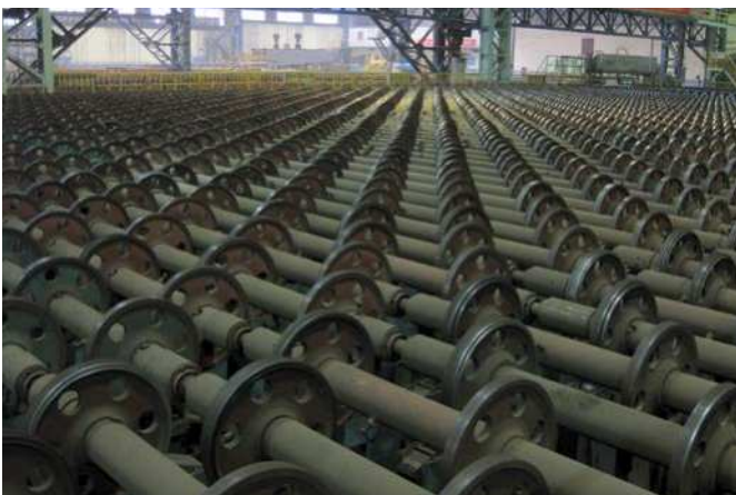
SKF DryLube bearings in the metal industry. Deep groove ball bearings in supporting rollers for cooling bed in hot rolling mill.
