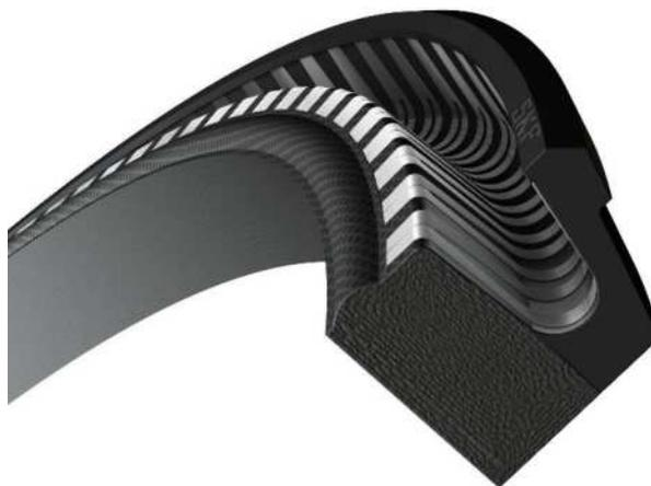
Designed for external sealing, the E11/BT seal has a flexible sealing lip made of elastomer and a back reinforced with high resistant textile rubber.
