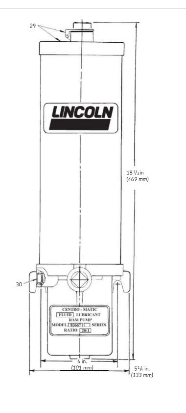
Use  $^3/8$  in.  $(9,5 \, mm)$  diameter mounting screws
