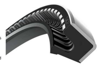
A vulcanized finger spring provides a uniform distribution of pressure on the shaft exerted by the sealing lip.
