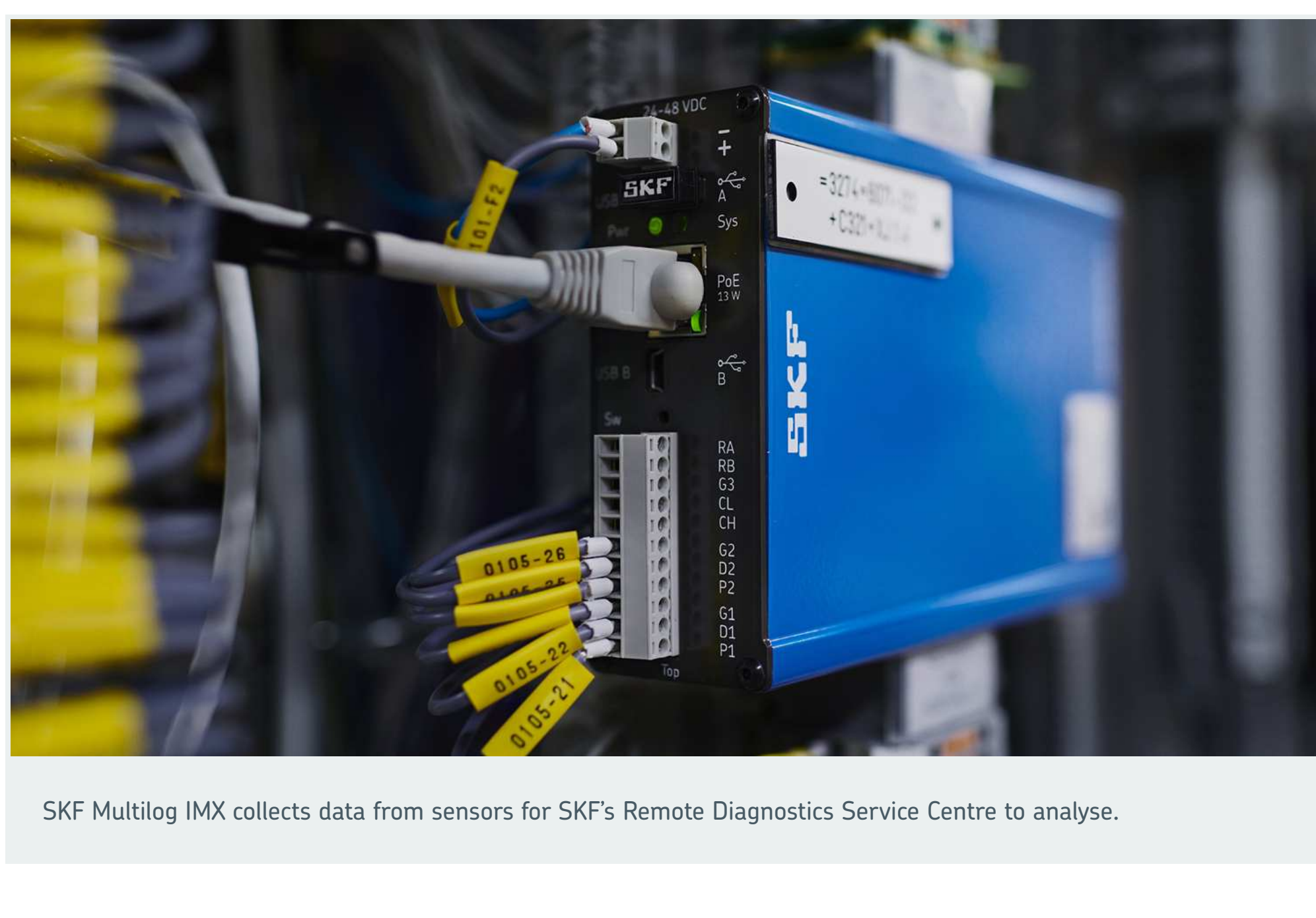
SKF Multilog IMX collects data from sensors for SKF's Remote Diagnostics Service Centre to analyse.
