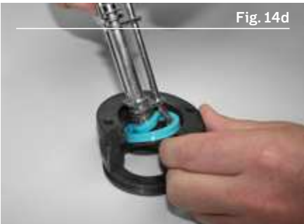
Inserting the seal into the housing
