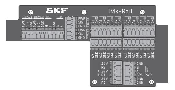
**Digital/tacho input connections D1 to D4** The digital input channels D1 to D4 support common types of two-, threewire tacho sensors. For each input, 3-terminals are available:
